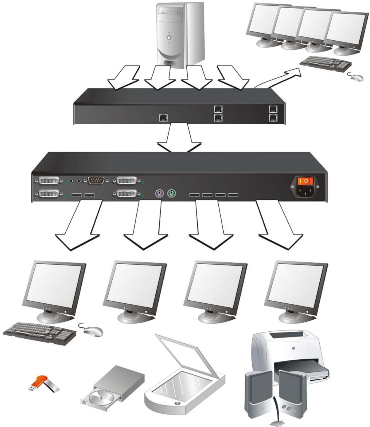
**DVI-D CATx KVM-Extender – with full USB 2.0 high speed access**
