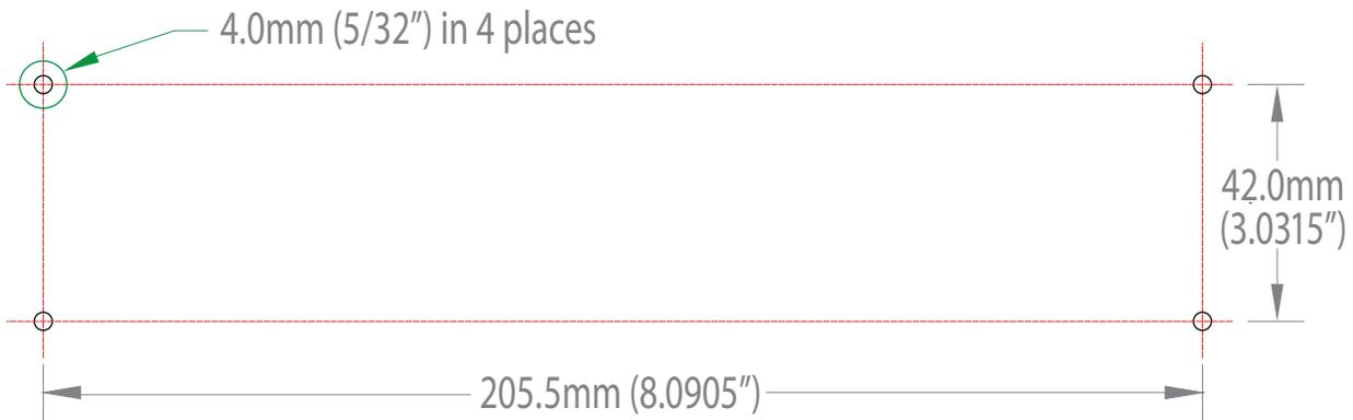
FIGURE 4-3. DIRECT SURFACE MOUNTING MEASUREMENT STENCIL
