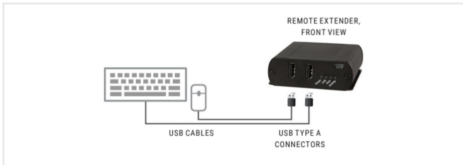
Attach your USB device(s) to the Remote Extender.
