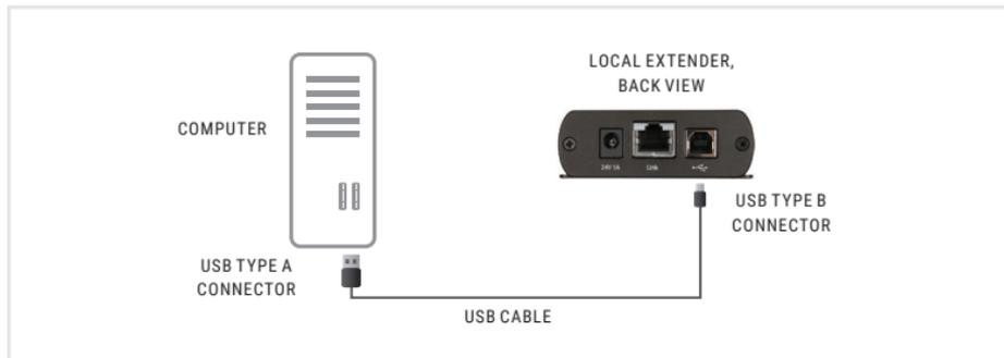
Connect the Local Extender into your computer using the included USB 2.0 cable.
