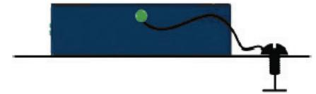
Figure 5. Grounding the chassis.
